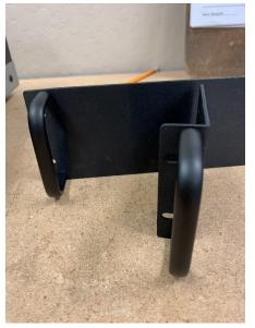
3. Attach the rack mounts to the DG645 and secure them with the screws that you've removed from the instrument in step 1.
